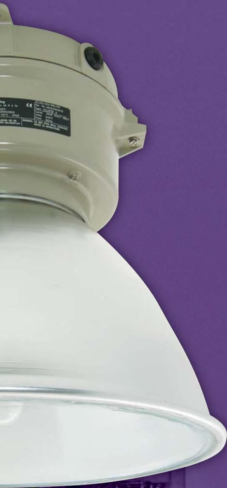
The Eclipse II incorporates unique features designed to make installation and maintenance quicker and easier. The lamp chamber utilises the restricted breathing Ex nR concept and lamp access is by means of the screwed cover glass, whilst the control gear area is separated from the lamp chamber by a barrier and is non sparking Ex nA, meaning that no special cable glands are required.
