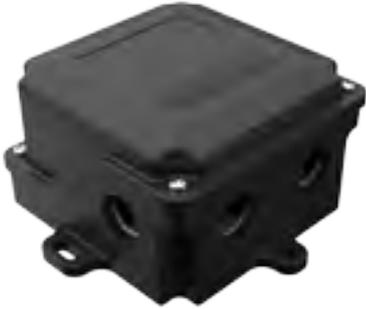
Hawke's range of Plastic Enclosures offer an operating temperature range from -60°C to +75°C with one-piece captive silicone gaskets offering excellent ingress resistance of up to IP66, IP67 and DTS01 deluge protection.
